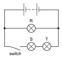
When the switch is open, which lamp(s) are not lit?
